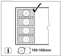
Place the cookware with the bottom diameter larger then 160 mm centrally between two sections
