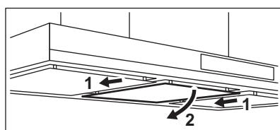
2. Slightly tilt the front of the filter downwards, then pull.
