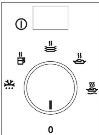
The control panel has a selector and an on/off switch. The control panel is only visible when the drawer is open.
